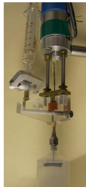
Fig. 3-3 Mechanical stirrer inside the driven syringe (at bottom) filled with sphere suspension. Small impeller at top of syringe is motorized through O-rings. Sphere suspension flows out through left side channel.
