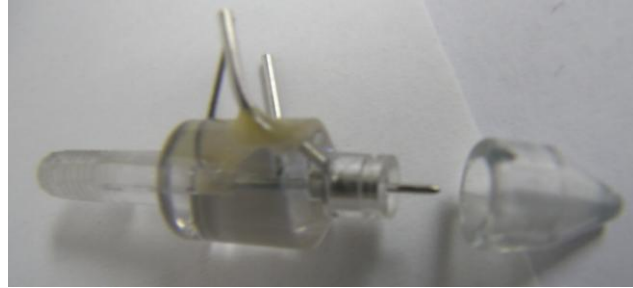
Fig. 3-6 A BD flow cytometer injector and nozzle with 80 \mu\text{m} I.D. sapphire orifice in the apex of the nozzle. Core fluid enters the furthest left tube and has a carefully machined tip on other end. Other two tubes are for sheath fluid and de-bubbling.
